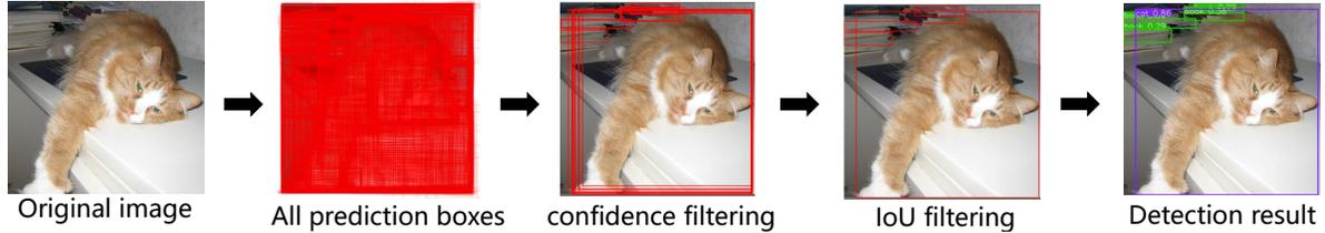
Figure 9. Visualization of the entire NMS process: a) original image; 2) pre-processed results with all the prediction boxes; 3) box filtering with confidence threshold; 4) additional filtering with IoU threshold; 5) Final detection result.
